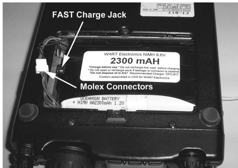
**NOTICE: DO NOT** use any conductive tool (e.g., screwdriver, knife, ...) in the installation of your OPP. **DO NOT** insert anything into the OPP+ power jack other than the proper size and type plug. If you violate these instructions, you can damage the battery pack and the warranty will be void.
