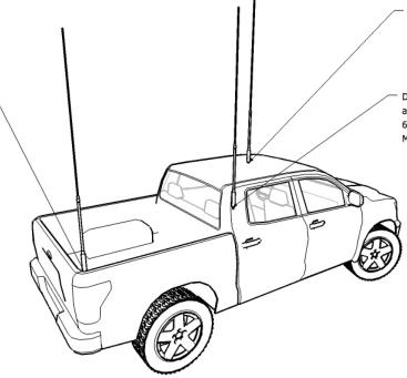
Rooftop installation with Mag-Mount: A secondary ground wire will be needed to ground the coax shield to the vehicle chassis or frame. The ground wire as to be as short as possible. The UNUN must be installed within 6" or less of the antenna with the red tip oriented toward the mount. The closer the better.
