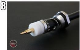
Insert the second teflon disc as shown in the picture.
