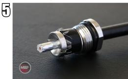
Flatten the wires as shown in the picture and cut the excess.
